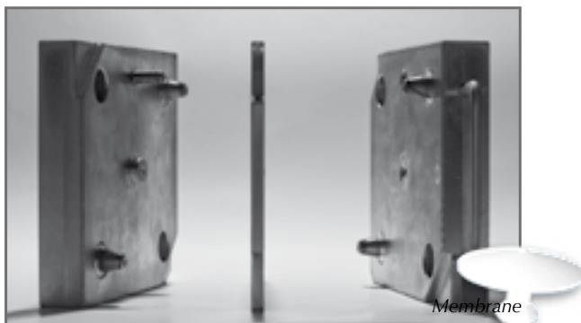
Prototype mold, 3 plates, 1 cavity, of a membrane
